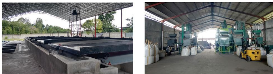
Figure 9: Processing plant – (left: shaking table, right: electrostatic & electromagnetic separators)
