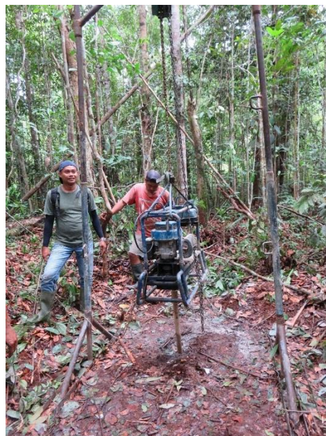
Figure 3-5 Mechanical auger drill used during phase 2
