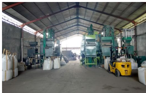
Exhibit 2.13: Electrostatic and Electromagnetic Separators Installed at the PTIM Plant
