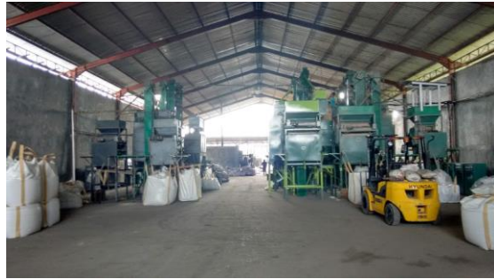
Figure 6-2 Electrostatic and electromagnetic separators installed at the PTIM plant
