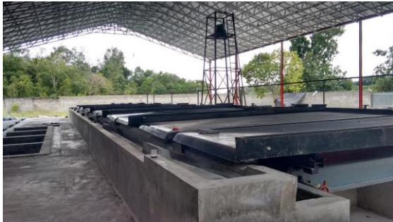
Figure 6-1 Shaking table at the PTIM plant
