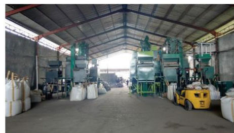
Figure 12: Processing plant – (Left: shaking table, Right: electrostatic & electromagnetic separators)
