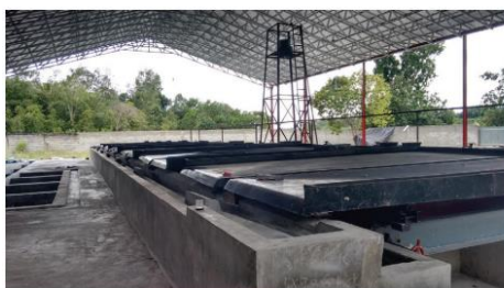
Figure 12: Processing plant – (Left: shaking table, Right: electrostatic & electromagnetic separators)
