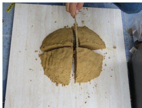
Figure 3-8 Cone and quartering of samples
