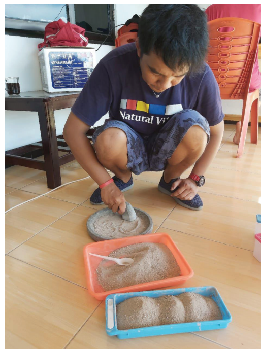
Figure 4-17 Drying and pulverising the samples
