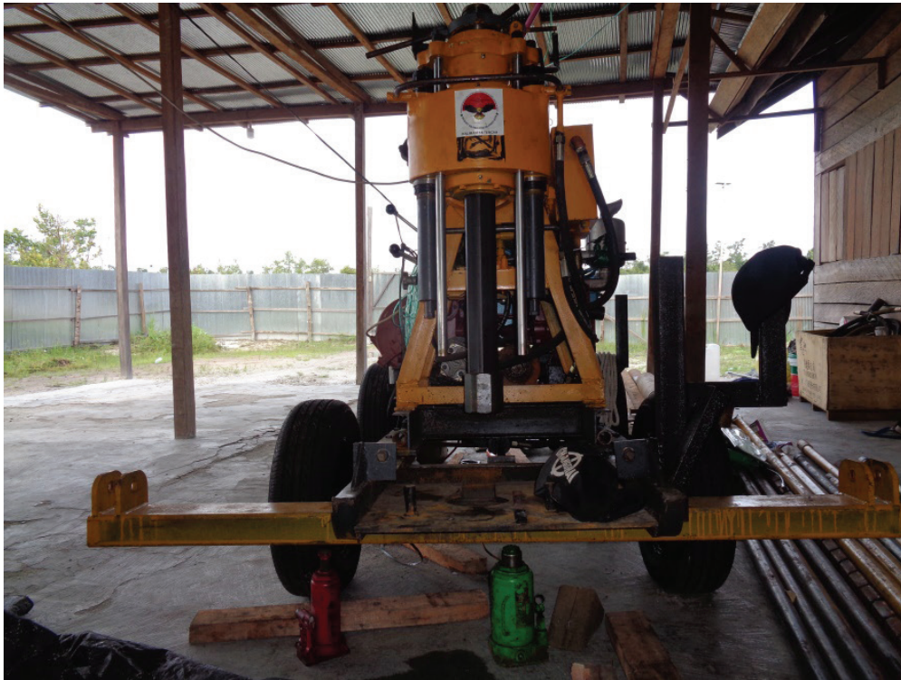
Figure 4-11 DP-180YY Drilling rig used for the resource drilling
