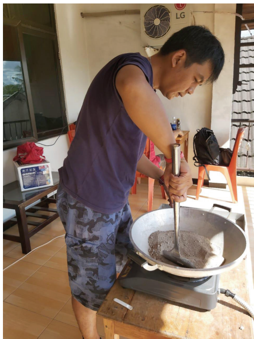
Figure 4-17 Drying and pulverising the samples
