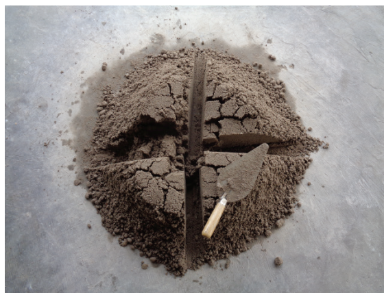
Figure 4-18 Example of cone and quartering
