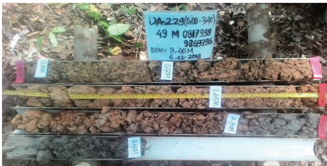
Figure 3-9 Core from auger hole DA-229 laid out for logging
