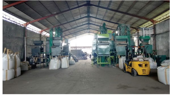
Figure 3-22 Electrostatic and electromagnetic separators installed at the PTIM plant
