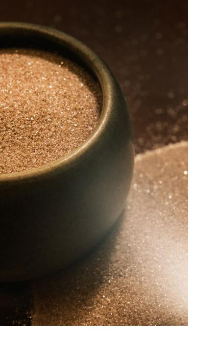
As a raw material in ceramic glazes, increasing the zircon content enhances the resistance to corrosion and chemical attack. In advanced ceramic applications, such as the production of biocompatible ceramics, zircon is used as a raw material for the production of fused and chemically derived zirconia.
