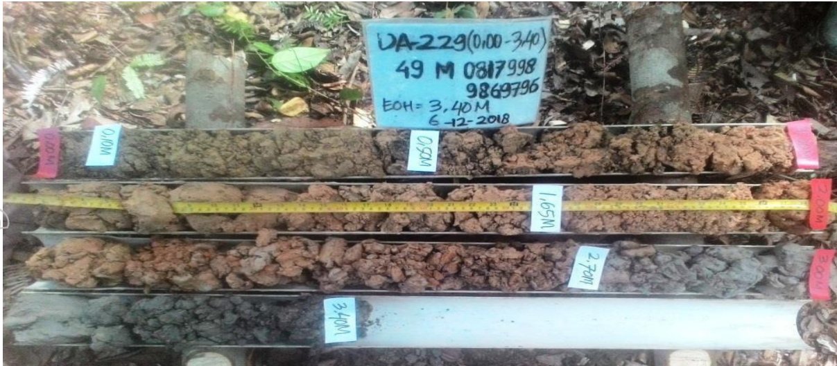
Figure 3-6 Core from auger hole DA-229 laid out for logging
