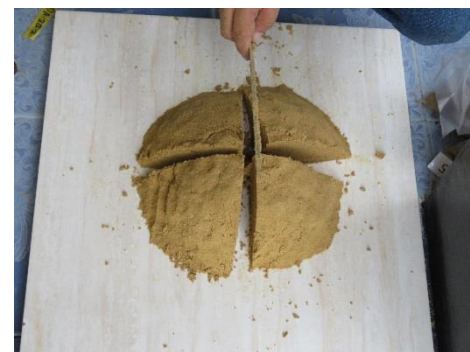
Figure 3-5 Cone and quartering of samples
