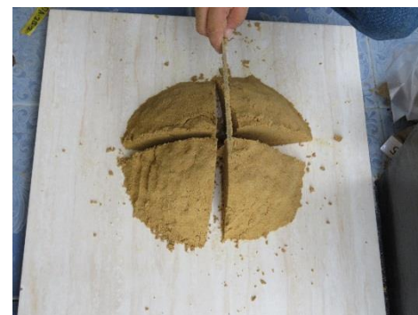
Figure 3-5 Cone and quartering of samples
