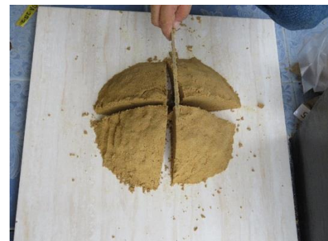
Figure 3-5 Cone and quartering of samples
