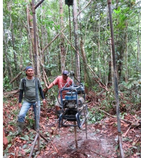
Figure 3-4 Mechanical auger drill used during phase 2
