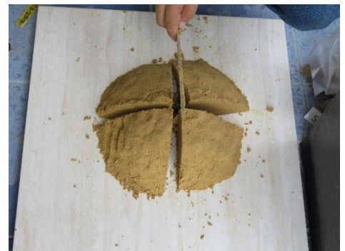
Figure 3-5 Cone and quartering of samples
